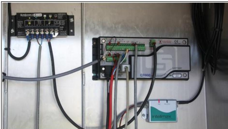
Figure 7 - Datalogger, modem and solar regulator
