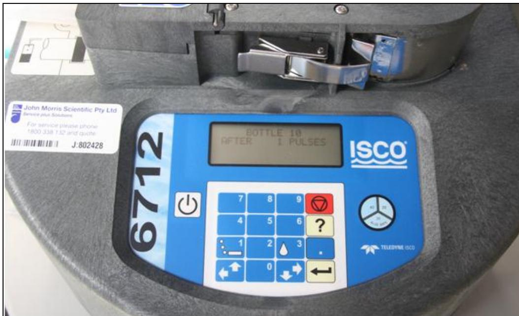
Figure 4 - ISCO automatic sampler
