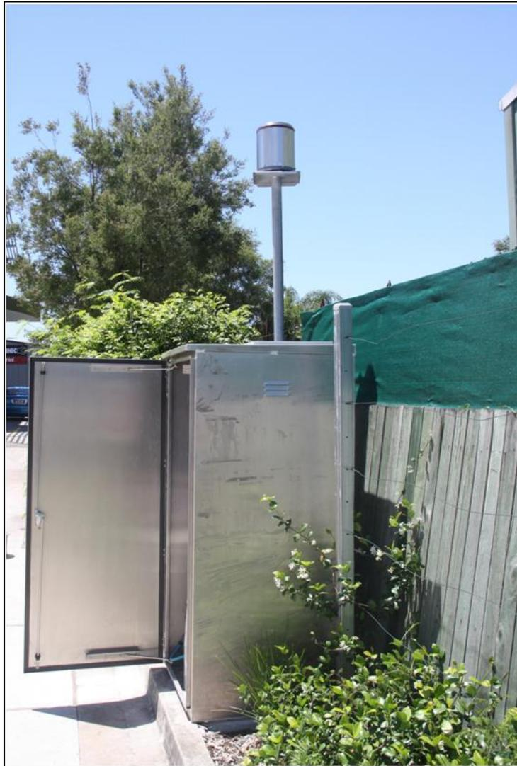
Figure 6 – Rain gauge mounted against cabinet
